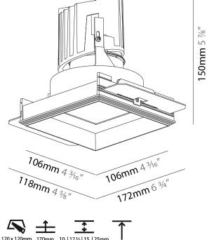
**120 x 120mm 170mm 10 | 12 ½ | 15 | 25mm** 4<sup>3</sup>/4" x 4<sup>3</sup>/4" 6<sup>1</sup>/<sub>16</sub>" <sup>3</sup>/<sub>8</sub>" <sup>1</sup>/<sub>2</sub>" <sup>9</sup>/<sub>16</sub>" 1"
